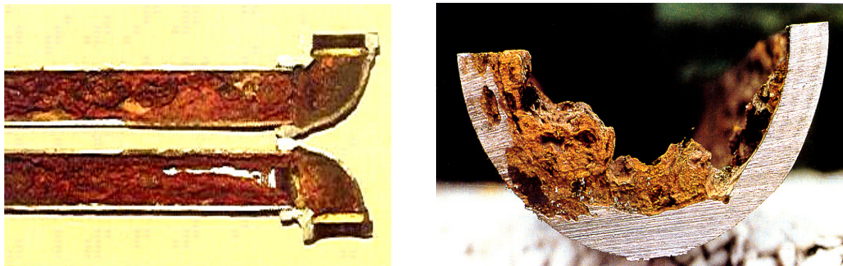
Figure.1 A general aging case for plumbing fixture
